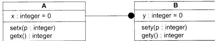
Diagram D.8 A one-to-many association (exactly two instances of class B may be associated with an instance of class A)
